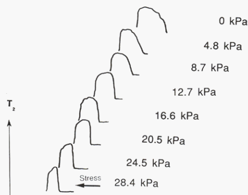
Figure 8. Intensity profiles from the ^1\text{H} T_2 enhanced image of PMAA gel as a function of stress.
